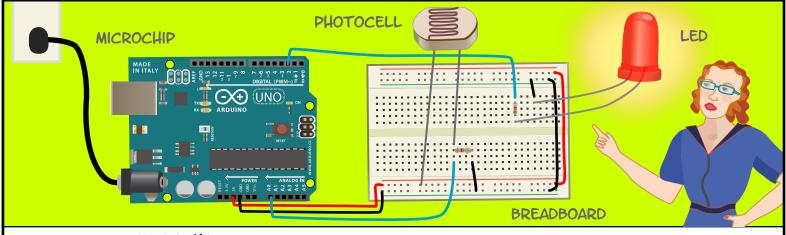
AN ARDUINO IS A **MICROCHIP**, WHICH IS A VERY SMALL COMPUTER THAT YOU CAN PROGRAM TO RESPOND TO THINGS. IT CAN MEASURE CONDITIONS (LIKE HOW MUCH LIGHT THERE IS IN THE ROOM). IT CAN CONTROL HOW OTHER OBJECTS REACT TO THOSE CONDITIONS (ROOM GETS DARK AND AN LED TURNS ON).
